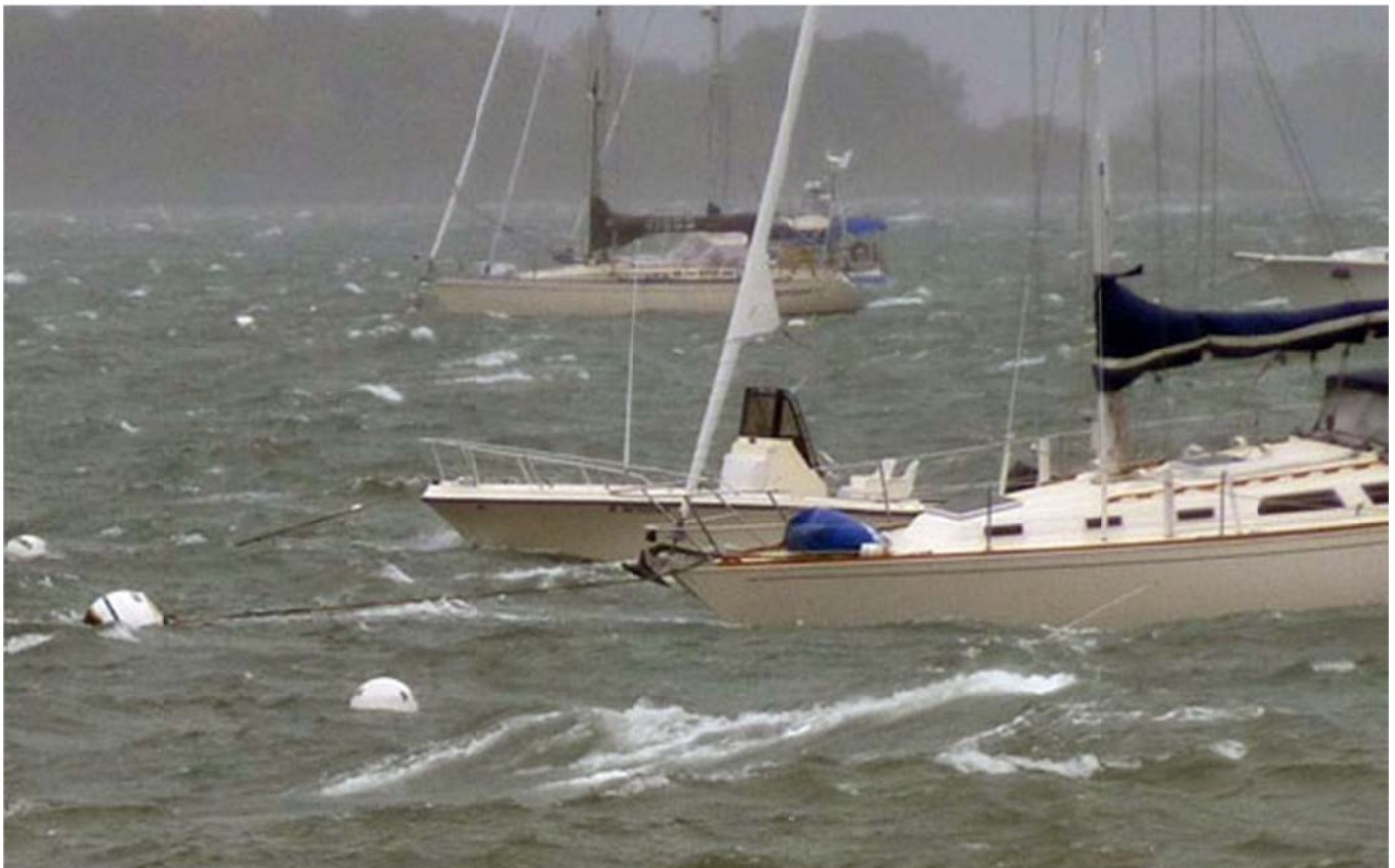
Elastic mooring rode and storm pendants can provide a reduction in jarring impacts under severe storm conditions (photo from ecomooringsystems.com )
