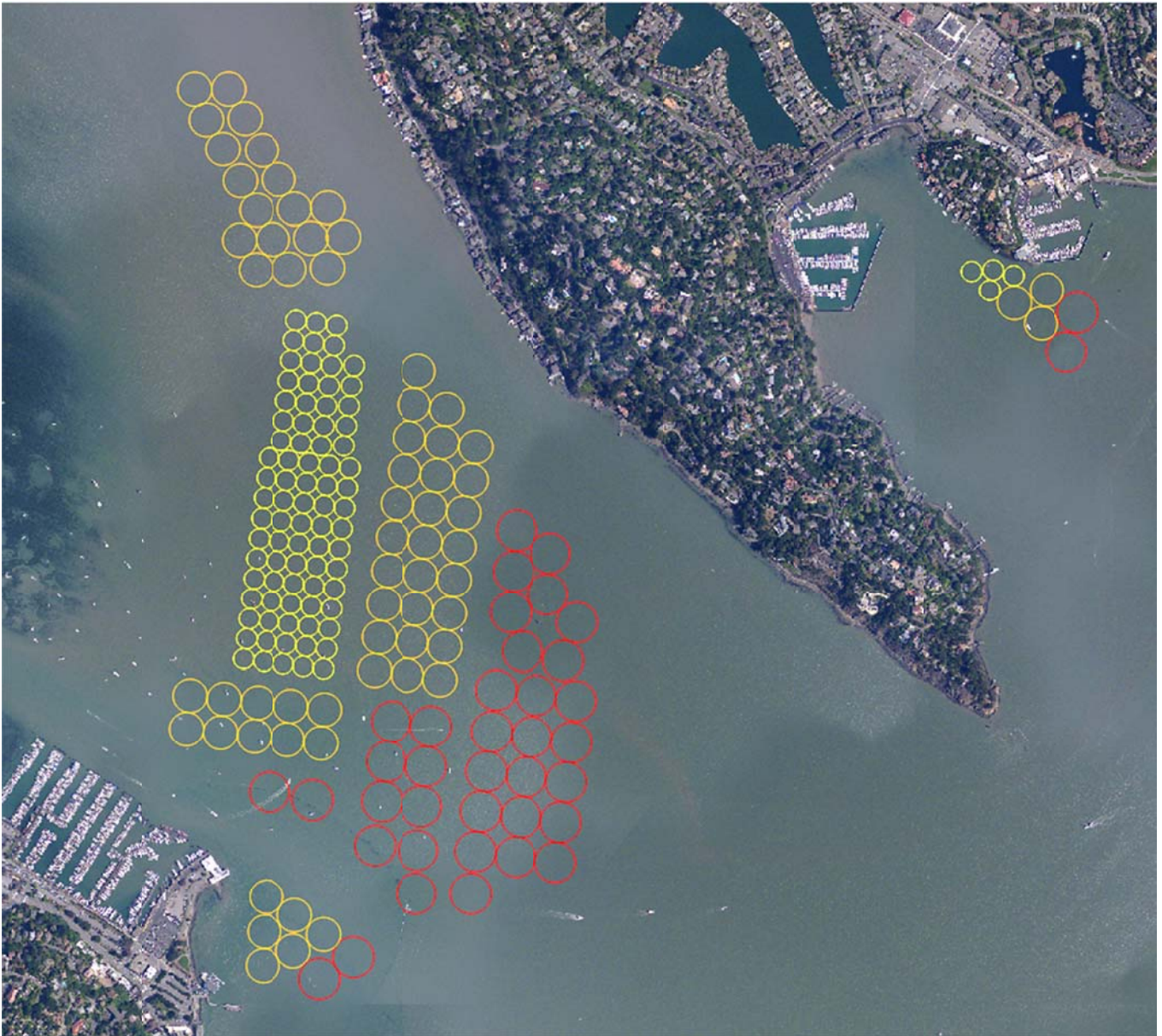
Example configuration of moorings using extremely large radii of 75 feet (yellow), 125 feet (orange), and 150 feet (red). The tight packing of moorings with these larger than required radii demonstrates that capacity for mooring positioning exceeds need or desirability of any of the stakeholder parties. As such considerable flexibility would exist for scaling and adapting mooring locations to address concerns beyond the scope of the present study.
